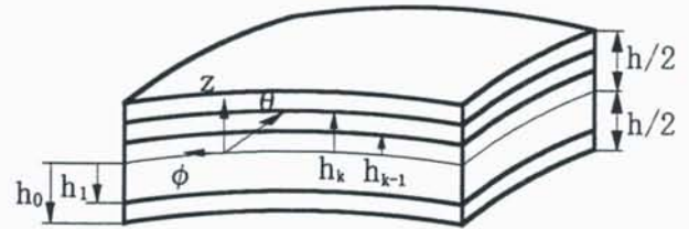
Fig. 2 Cross-sectional view of shell
