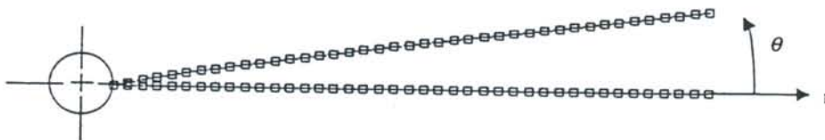
Fig.2: An axisymmetric circumferential vibrating mode (in-plane torsional mode), \bar{\omega} = 6.568 , for C-F boundary condition, b/a=0.1 , a/h=10 and \bar{\Omega} = 4 ( u=w=0.0 )
